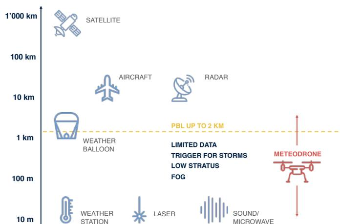
Figure 1: Meteodrone closes the data gap.
