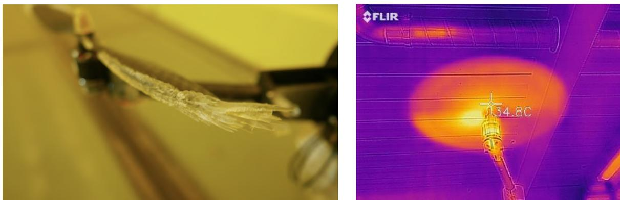
Figure 7: Extreme accumulation of clear ice amount (left) and heating of propellers (right).
